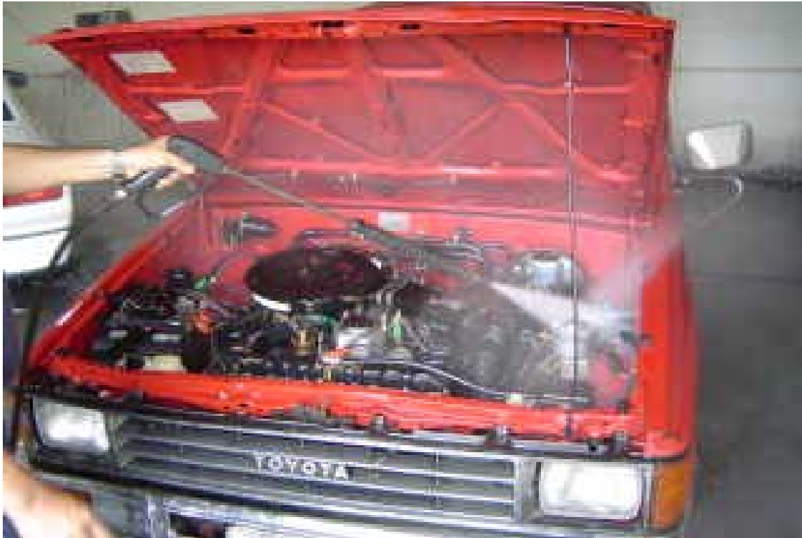
Figure 2-2. Detailer Applying Water-Based Cleaner with High Pressure Wand.
