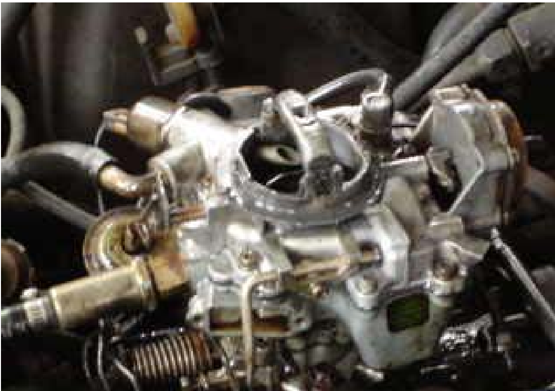
Figure 2-10. Carburetor Cleaned with Low-VOC Cleaners.
