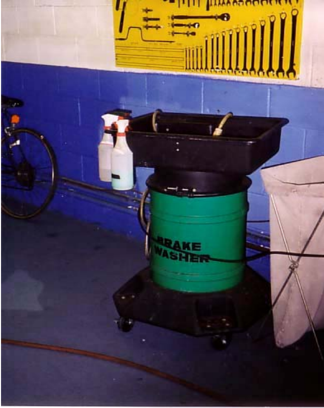
Figure 2-8. Parts/Brake Cleaning System.
